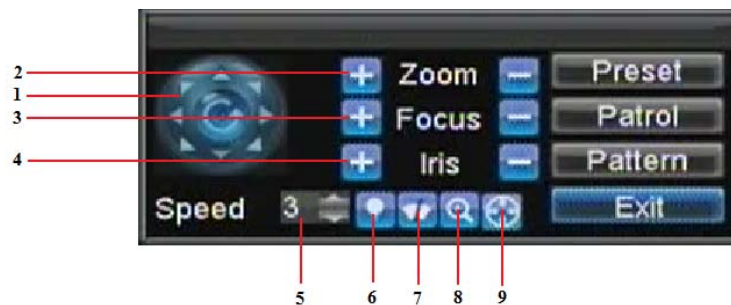
Figure 3. PTZ Control Interface
